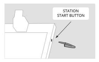
Press the start button with a nonsharp, non-pointed tool like a pen cap to turn on the station
